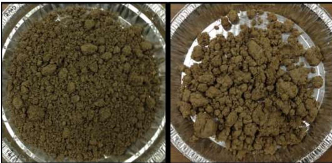
Figure 2. Photographs of point bar soil sample (left) and undercut bank sample (right) after drying. Soil in the undercut bank shows more cohesion and has formed more aggregates that are also larger in size.
